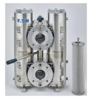
The duplex configuration of the ASME certified stainless steel pressure filter from the **EDA range** can be used for continuous operation: If a filter element has to undergo maintenance, or the element must be replaced, the operator can redirect the flow through the filter from one side to the other.
