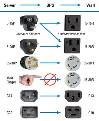
Notes: UPS models 1500 VA and below plug into a standard 15A or 20A wall socket. R = Receptacle, P = Plug, L = Locking
