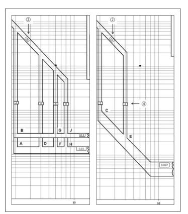
Figure 2. Flat response SD profiles (left) and I<sup>2</sup>t response SD profiles (right)
