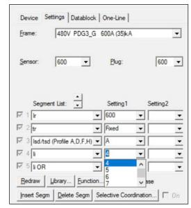
Figure 7. Selecting the I, (continuous current) rating
