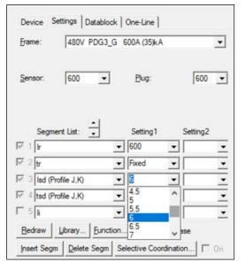
Figure 14. Setting the Short Delay Pickup  $(I_{sd})$  to a custom value
