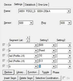
Figure 12. Setting Segment 5 to Instantaneous Pick-up (I<sub>i</sub>)
