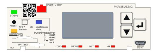
2.2 PXR 25, PXR 25 Motor Protection, and 20D display with keypad
