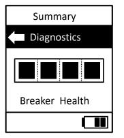
When the summary of life is indicating 25% or less, the breaker should be inspected for possible replacement.
