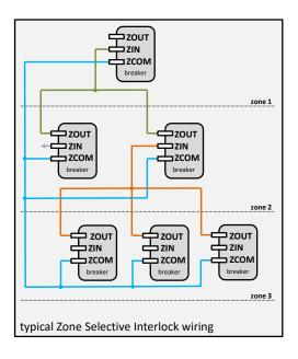
Motor protection circuit breakers are used in the final breaker (lowest zone) in a complete ZSI enabled system. The zone out (Zout) signal is sent whenever a short circuit delay protection or ground fault protection pickup is exceeded. This indicates to the circuit breaker in
