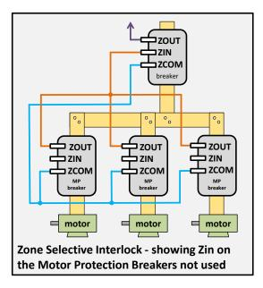
PXR trip units with a display have a visual indication of the ZSI system being active and connected to the other breakers in the ZSI system. A small check-mark will appear next to the ZSI when the trip unit receives a ZSI-IN signal. The general-purpose, configurable, relay contacts may also be programmed to indicate ZSI signals and status.
