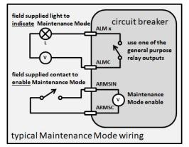
There are three ways to actuate the Maintenance Mode function, locally, remotely using a contact, or remotely using communications. A blue LED on the trip unit always illuminates to confirm when the function is enabled.
