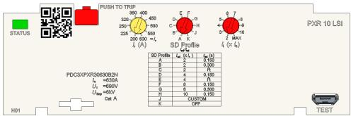
The PXR 10 trip curve configuration is simple, using the switches on the front panel. LSI trip units have three rotary switches, while the LI version has only two, eliminating the center "SD Profile" switch. For all, the yellow color rotary switch sets the  $I_r$  and the red switches define short circuit behavior. Details regarding the available protection settings for each frame are found in Section 9: Available protection settings.
