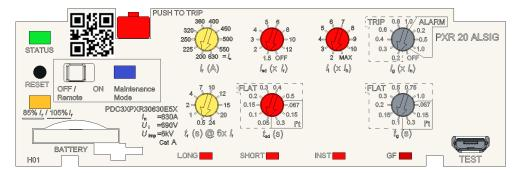
Depending on the trip unit style, up to seven rotary switches can be found on the trip unit's front panel. The switches are color-coded and set protection settings using a surrounding legend indicating the value of that setting. These are the core protection settings, other configurable settings can be set using PXPM. Details regarding the available protection settings.
