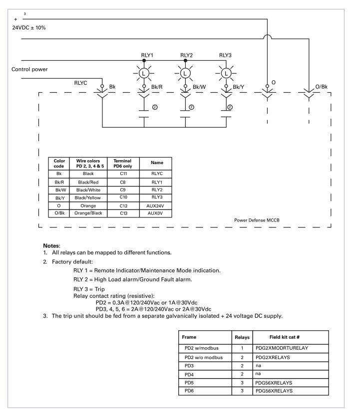
Auxiliary power and relay wiring
