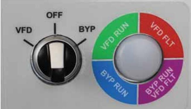
In the Bypass position, the VFD Keypad control is disabled and the motor started immediately in Bypass. This position also removes the RUN ENABLE input to the VFD (DigIn2).
