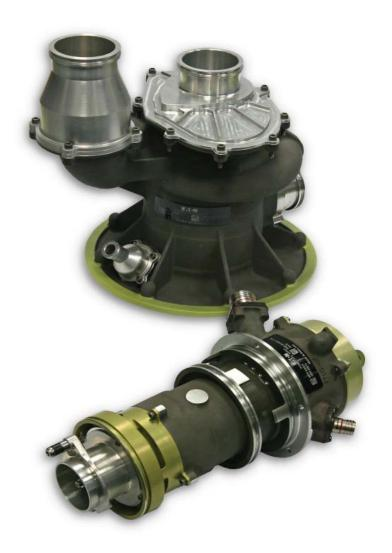
The Eaton designed 39-0001 boost pump is mounted within a 39-0004 canister installed in the aircraft fuel tanks. The pump incorporates a mixed flow impeller driven by an internal, fuel flooded, variable frequency 3 phase induction motor and provides fuel supply to the engines. The pump is capable of operation directly from a 200V L-L 360Hz to 800Hz three phase supply.
